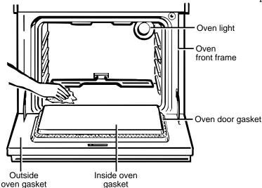
3. Clean spatters or spills on the oven front frame, and the oven door outside the gasket with a dampened cloth. The oven front frame and the oven door outside the gasket do not get cleaned by the self-clean cycle. On these areas use detergent and hot water or a soap-filled steel wool pad. Rinse well with a vinegar and water solution. This will help prevent a brown residue from forming when the oven is heated. Buff these areas with a dry cloth. Do not clean the gasket.
